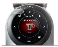
You can set the stand-by time in the programming menu. Press the **menu** key located above the display for 3 seconds.
