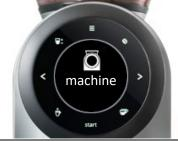
Select machine with the left/right arrow keys. Press start, and select automatic switch off. Press start and set the timing with the left/right arrow keys. (30 min, 1, 2, 4 hours, no switch off) Press start to confirm.
