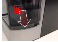
If the machine is not placed upright, the water outlet of the tank does not connect properly to the water inlet at the machine side. This will trigger a [flow error] message in the display.
